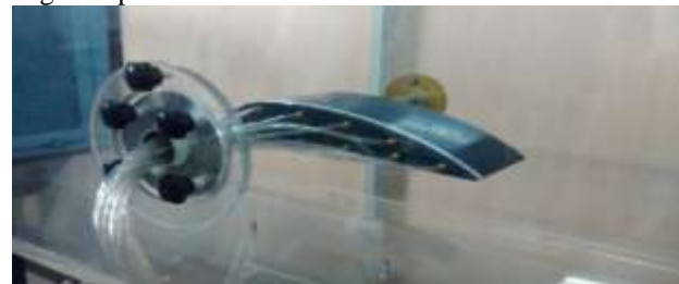
CROSS SECTION OF A SPOILER (INVERTED AIR FOIL)
